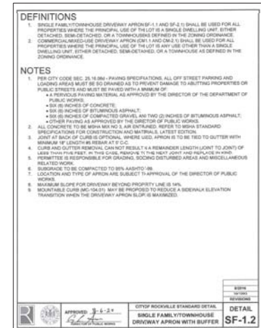
DETAIL H - SINGLE FAMILY/TOWNHOUSE DRIVEWAY APRON WITH BUFFER CITY OF ROCKVILLE STANDARD NO. SF-1.2
