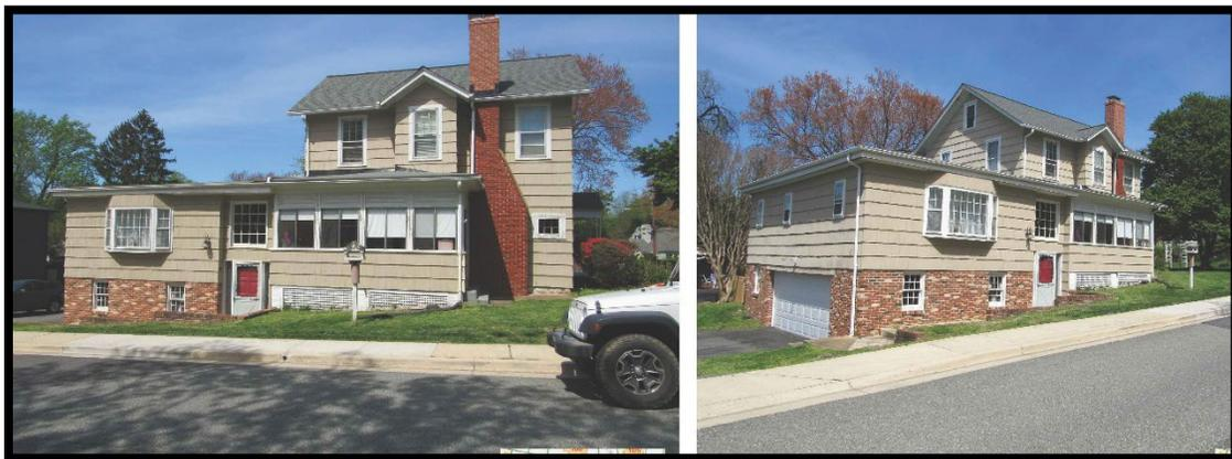
The west elevation of the existing addition has a double-wide garage door and a six-over-six double-hung window on the north end. Three six-over-six double-hung windows span the width of the second story. The original house has two evenly spaced second story windows, and an attic window in the peak of the gable. The proposed new addition will have three evenly spaced
